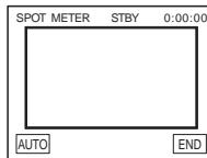
3 **Touch the point you want to adjust and fix the exposure on the screen.**
