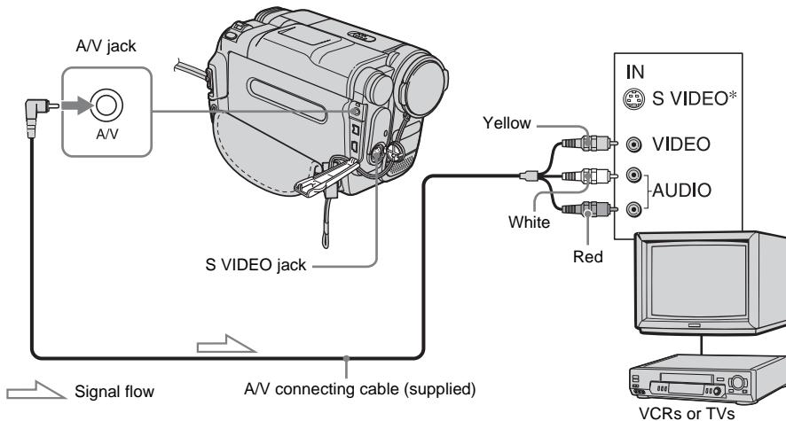
\* Pictures can be reproduced more faithfully by using an S video cable (optional). When there is an S video jack on the device to be connected, connect the S video plug to that jack instead of using the yellow video plug. The audio will not be output when you connect with the S video plug alone.
