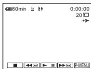
If the tape counter is not displayed, press **DISPLAY** on the Remote Commander.
