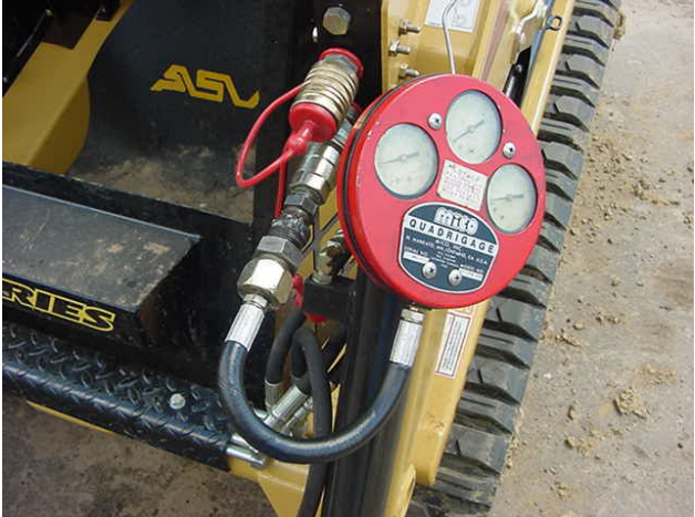
Figure 14-3 14-110 Insert the hydraulic gauge into one of the attachment quick couplers.
