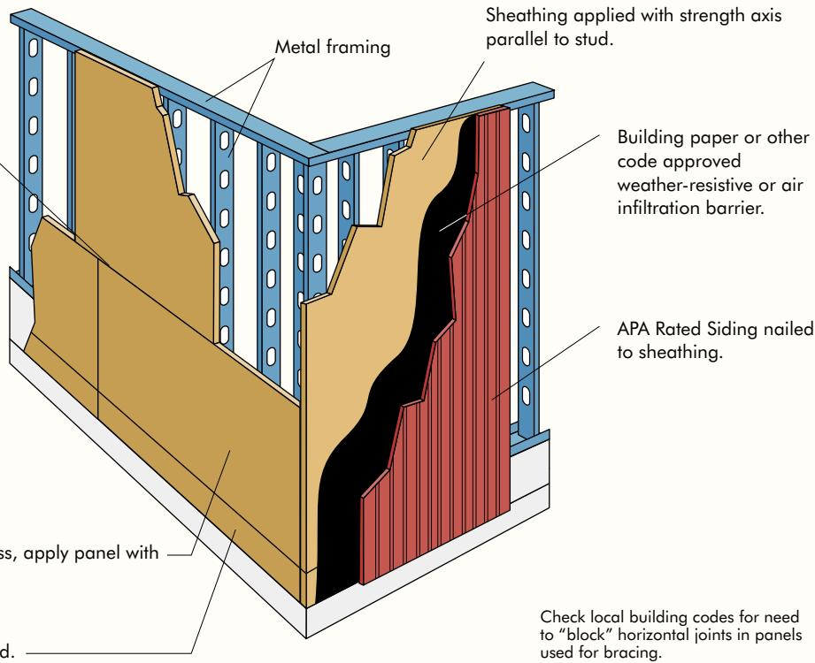
For extra sheathing stiffness, apply panel with strength axis across studs.
