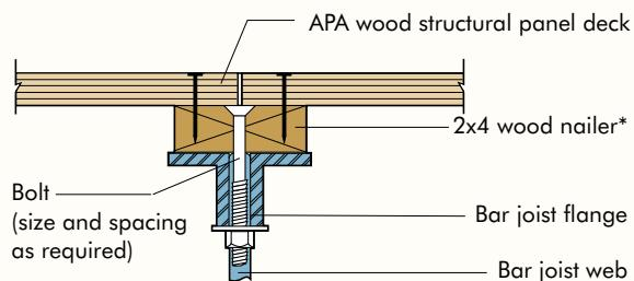
\*Nailers installed across joists are suggested where non-modular spacings are used.
